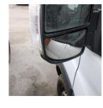
Door Mirror Glass ns Broken Needs Replaced Replace
