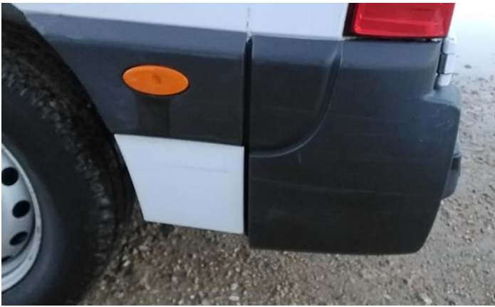
9: Qtr Panel nsr Dented With Paint Damage
