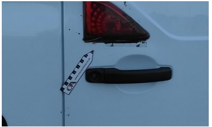
10: Qtr Panel nsr Dented With Paint Damage
