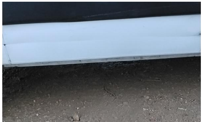
16: Qtr Panel osr Scratched Over 25mm Not Thru Paint
