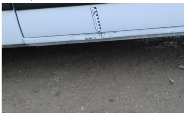
6: Door nsf Dented Over 2 UpTo 10mm
