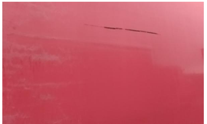
4: Panel Front Scratched Over 25mm Thru Paint
