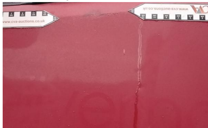
5: Door nsf Dented With Paint Damage
