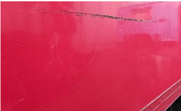
5: Roof Dented With Paint Damage
