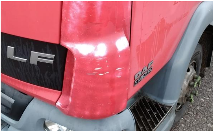
3: Bumper Front Cracked Over 25mm
