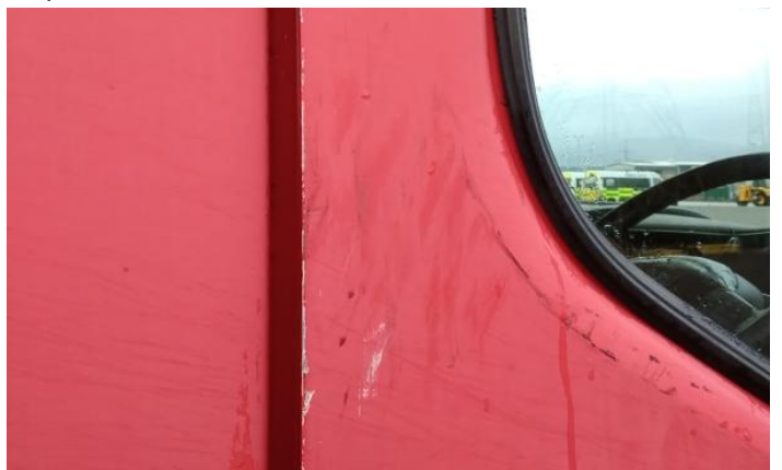
12: Qtr Panel osr Cracked Replace
