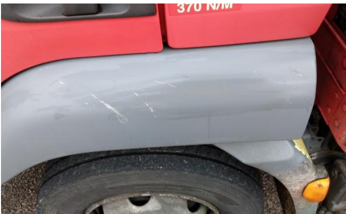
5: Bumper Front Moulding Scratched (Painted) Over 25mm Thru Paint
