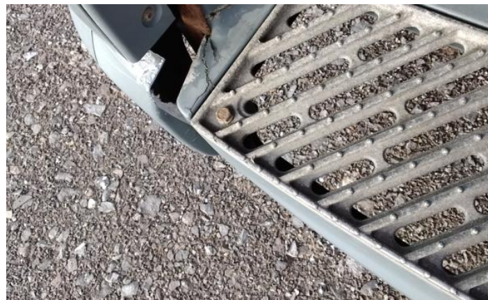
3: Bumper Front Dented Over 30mm
