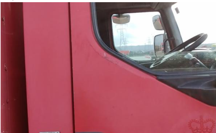
5: Moulding nsf Wing Broken Replace
