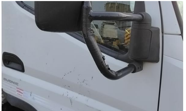
16: Door osf Chipped Edge Chip
