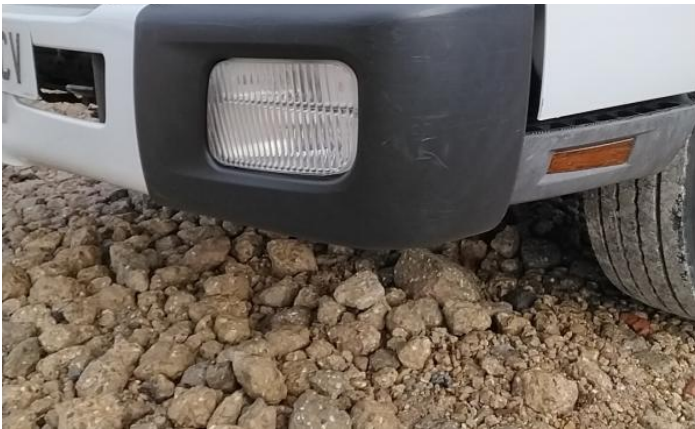
3: Bumper Front Dented Over 30mm
