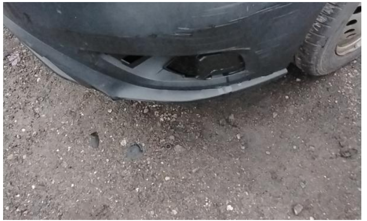
4: Bumper Front Moulding Missing Replace
