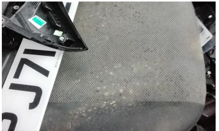
18: Seat Back Cover osf Holed Over 3mm
