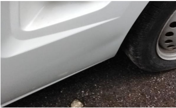
9: Door nsf Dented With Paint Damage
