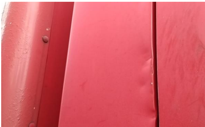
15: Seat Base Cover osf Holed Over 3mm
