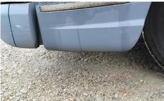
5: Bumper Front Scratched 25 to 100mm Thru Paint
