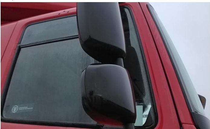
5: Wing nsf Cracked Replace
