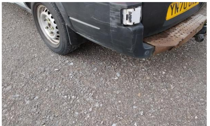
12: Panel Rear Scratched Over 25mm Thru Paint
