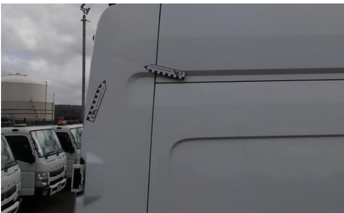
17: Door osr Dented Over 30mm
