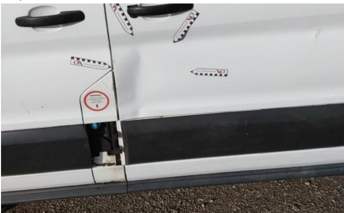
5: Aperture Seal nsf Broken Replace
