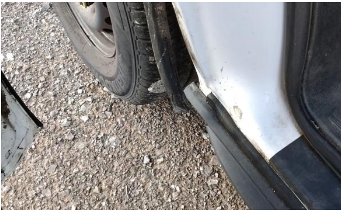
3: Wing Front Arch Extension ns Broken Replace
