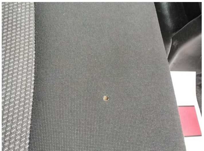
8: Seat Base Cover osf Holed Over 3mm
