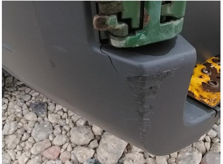
4: Bumper Rear Moulding Broken Replace
