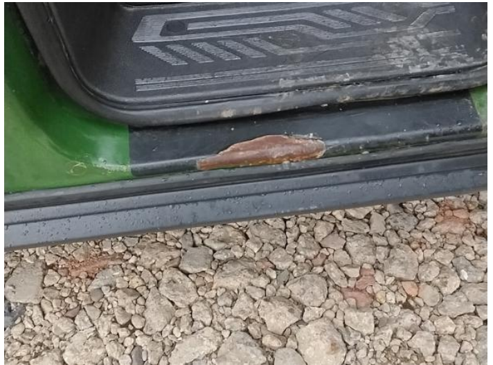
6: Sill ns Rusted Over 5mm
