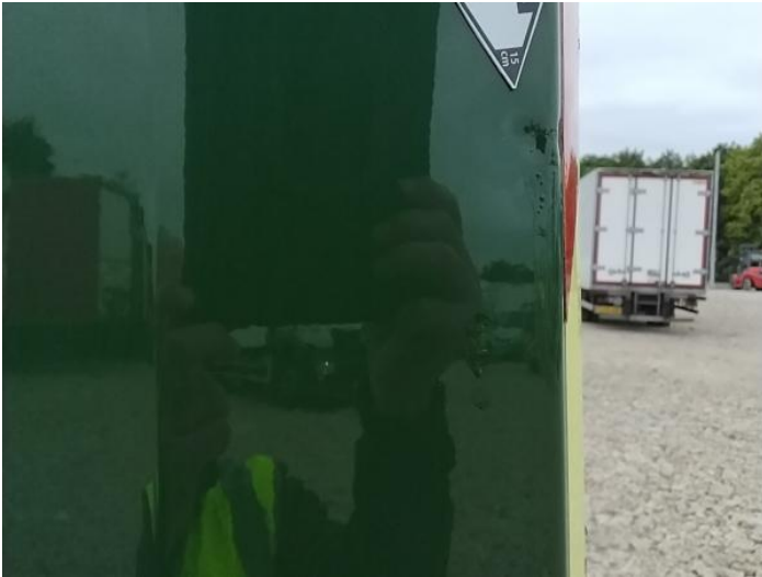
3: Panel Rear Dented Between 10mm + 30mm
