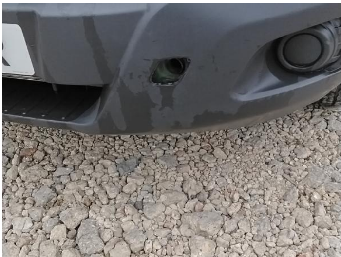
1: Front TowEye Cvr Missing Replace
