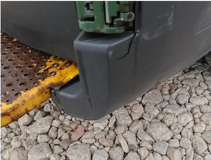
5: Bumper Rear Moulding Broken Replace
