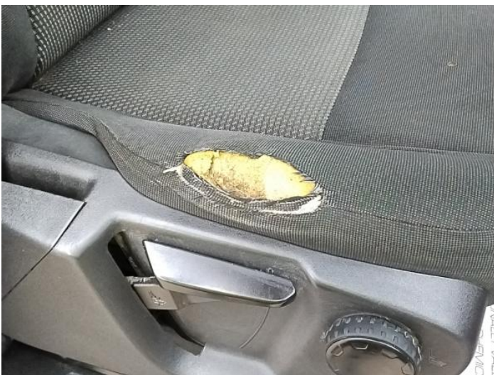
7: Seat Base Cover osf Holed Over 3mm
