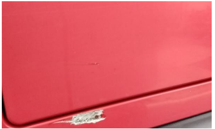
4: Bumper Front Dented With Paint Damage
