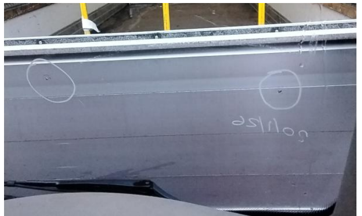
4: Door osf Scratched Over 25mm Thru Paint
