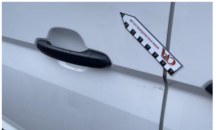
10: Qtr Panel nsr Dented With Paint Damage
