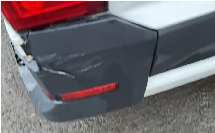
3: Sill os Dented With Paint Damage
