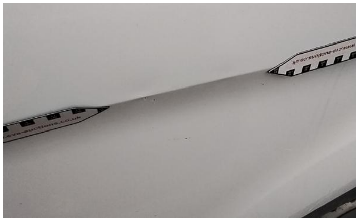
10: Door osr Dented With Paint Damage
