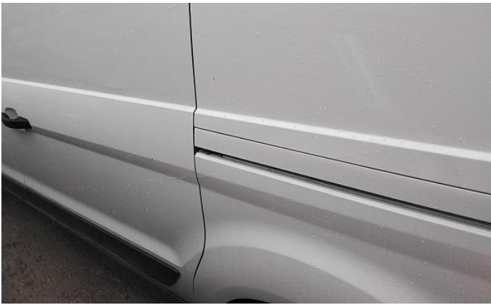
3: Door nsf Scratched Over 25mm Thru Paint
