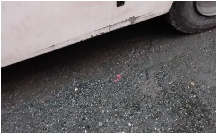
3: Door nsf Scratched Over 25mm Thru Paint
