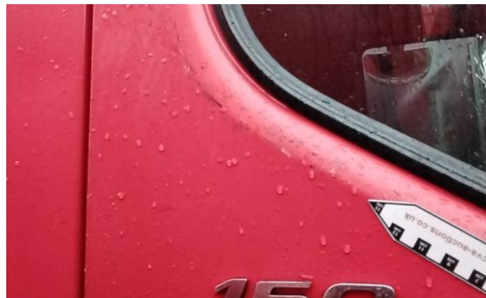
3: Panel Front Poor Previous Repair Rippled Up To 30%
