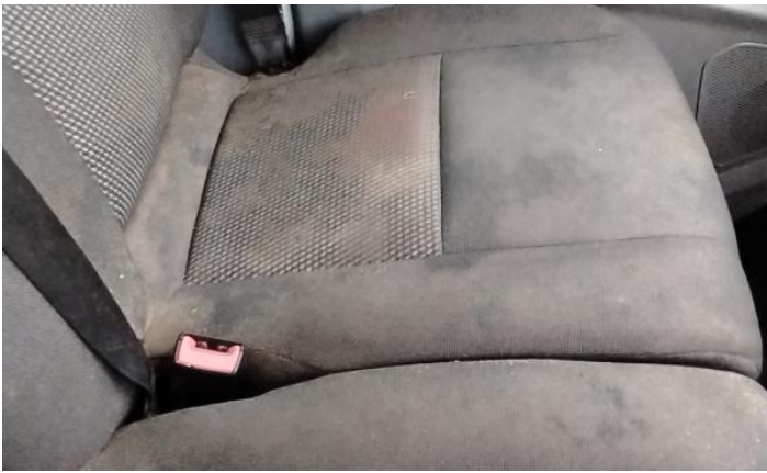
21: Seat Base Cover osf Holed Over 3mm
