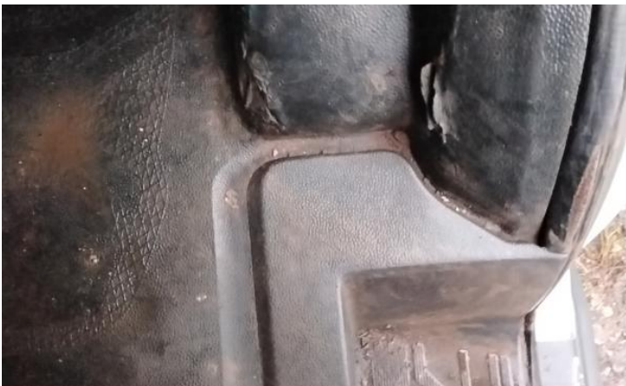
17: Door osf Chipped Multiple Chips
