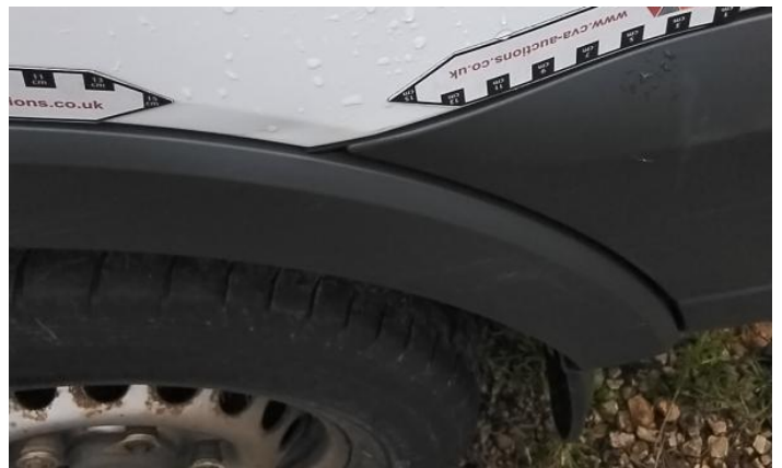
10: Qtr Panel nsr Dented With Paint Damage
