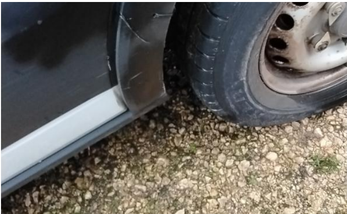
9: Qtr Panel nsr Dented With Paint Damage
