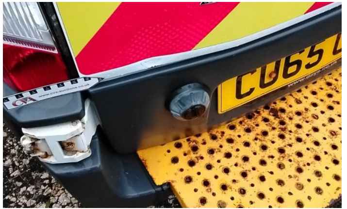
16: Qtr Panel Moulding ns Scuffed (Unpainted) Over 100mm
