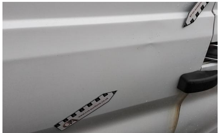
10: Qtr Panel nsr Dented Over 30mm
