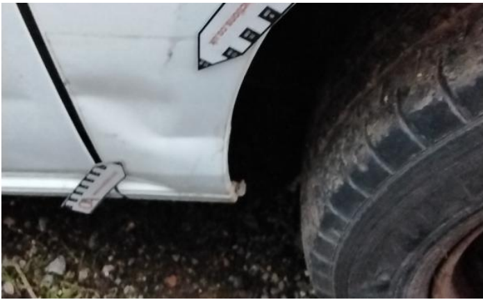
3: Qtr Panel nsr Dented With Paint Damage
