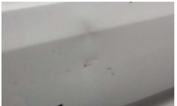
18: Qtr Panel osr Scratched Over 25mm Thru Paint
