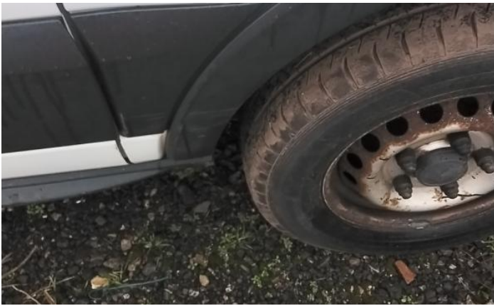
9: Qtr Panel nsr Dented With Paint Damage
