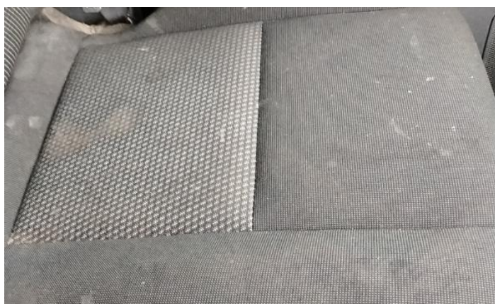
24: Seat Base Cover osf Holed Over 3mm
