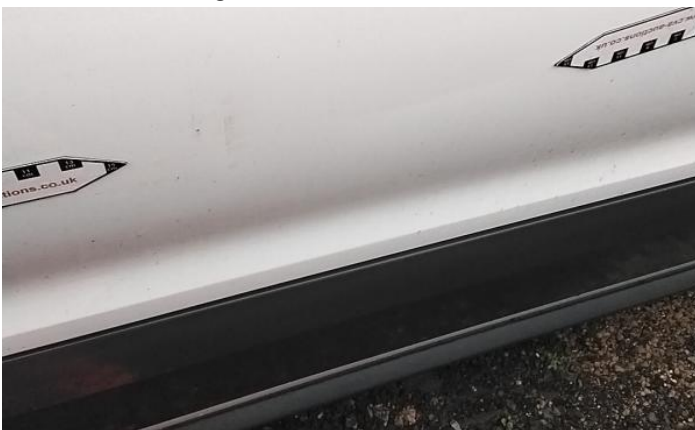
17: Door osr Dented With Paint Damage
