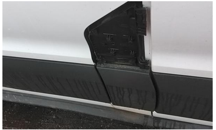
4: Door nsf Dented Over 30mm
