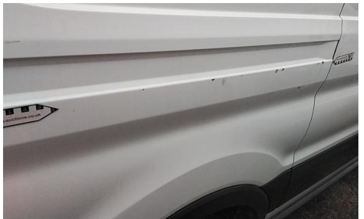
16: Door osr Dented With Paint Damage
