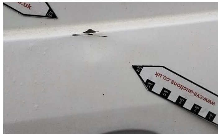
15: Door nsr Chipped Multiple Chips
