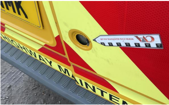
3: Qtr Panel osr Dented With Paint Damage
