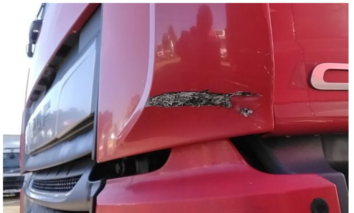
4: Screen Front Chipped Over 10mm
