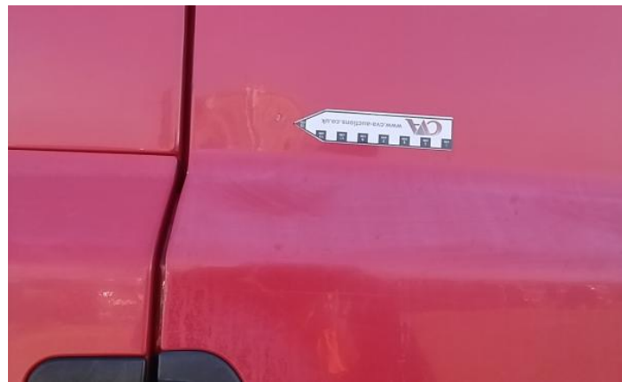
9: Door nsf Scratched Over 25mm Thru Paint
