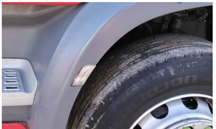
6: Wing nsf Chipped Multiple Chips
