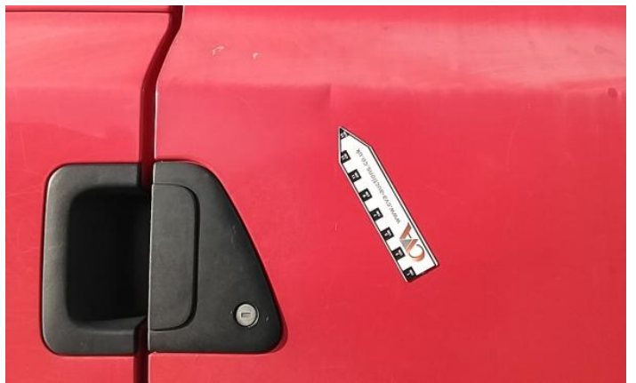
10: Wing Front Arch Extension os Scratched (Painted) Over 25mm Not Thru Paint
