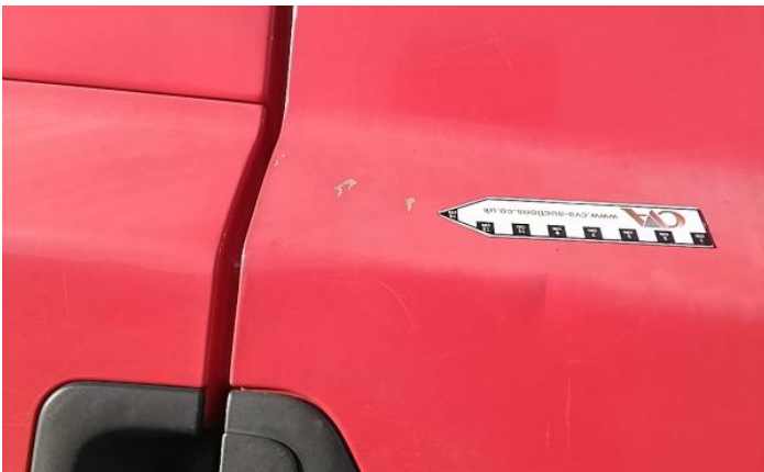
11: Door osf Dented With Paint Damage
