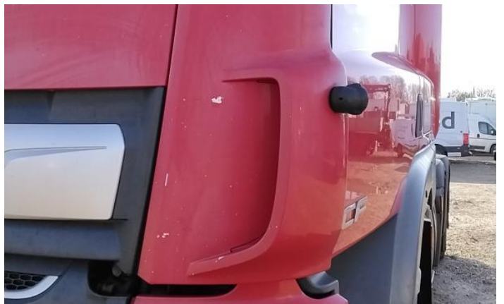
4: Screen Front Chipped Over 10mm
