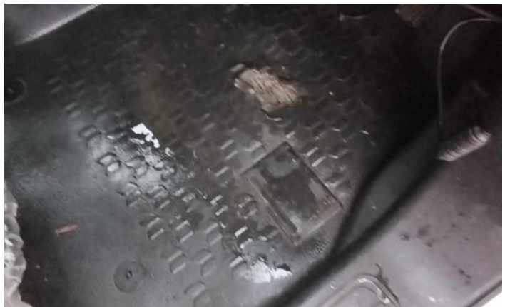
12: Seat Base Cover osf Holed Over 3mm
