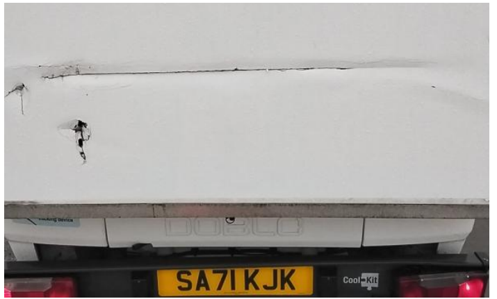
4: Wing nsf Dented With Paint Damage
