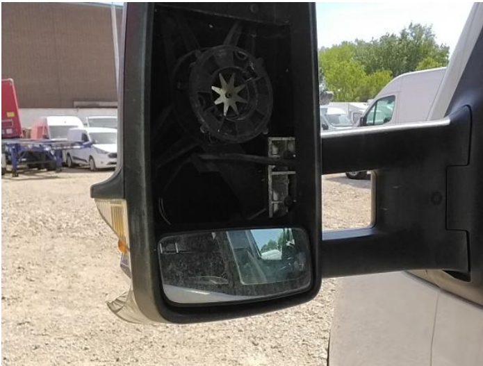
5: Door Mirror Glass ns Missing Replace
