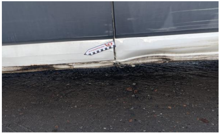
16: Qtr Panel nsr Dented With Paint Damage
