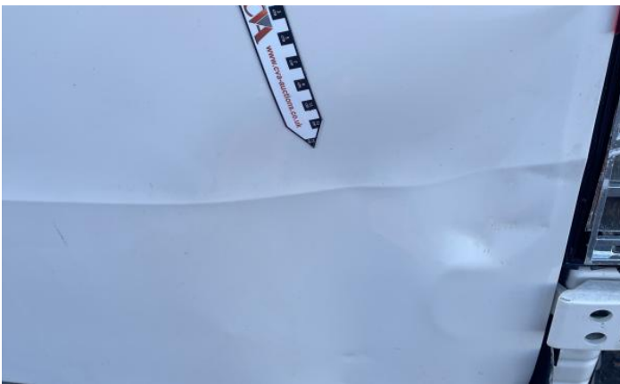
9: Qtr Panel osr Dented With Paint Damage
