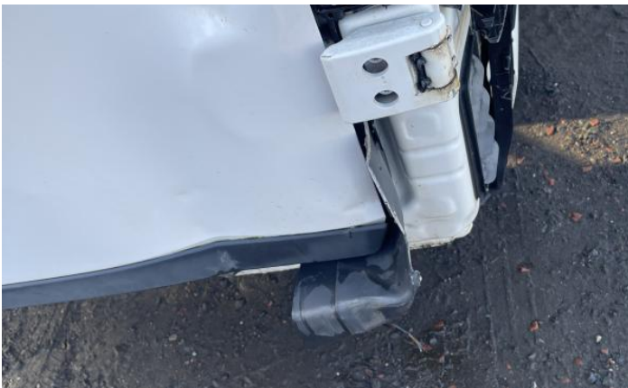
11: Tailgate Dented With Paint Damage
