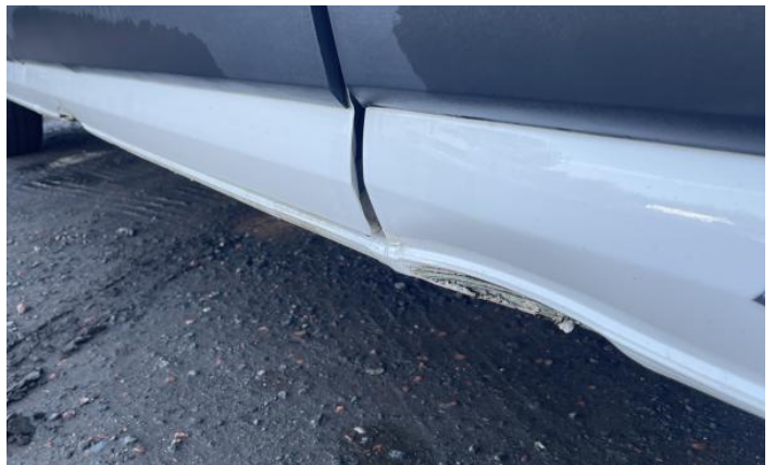
6: Qtr Panel osr Dented With Paint Damage
