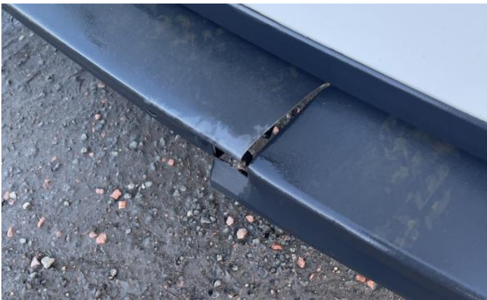
5: Qtr Panel Moulding os Broken Replace
