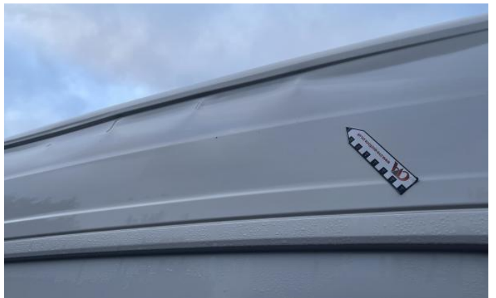
12: D Post ns Dented With Paint Damage
