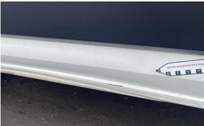
5: Door osf Dented Over 2 UpTo 10mm
