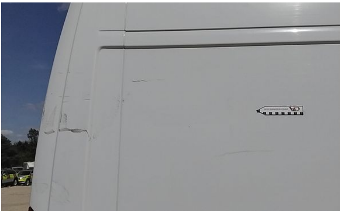
11: Door osr Dented Between 10mm + 30mm
