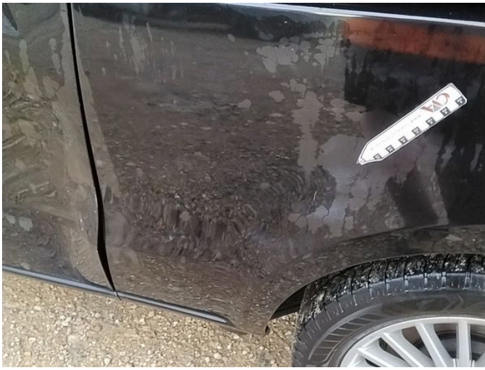
4: Qtr Panel nsr Dented Over 30mm
