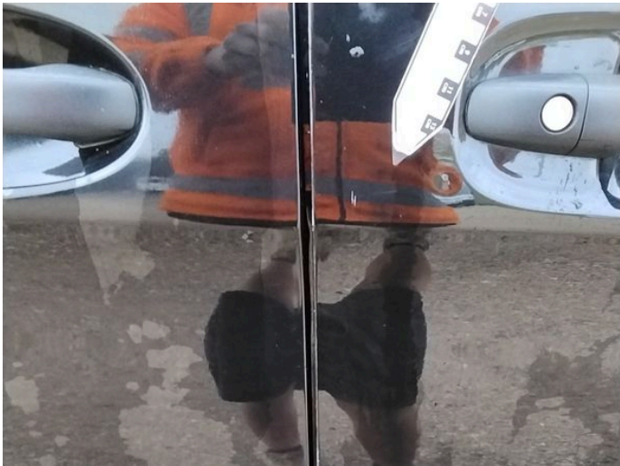
7: Door osf Scratched UpTo 25mm Thru Paint
