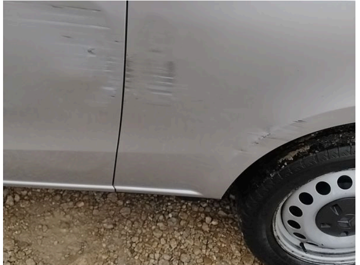
2: Qtr Panel nsr Dented With Paint Damage
