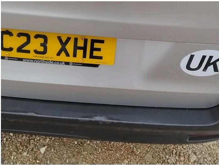
4: Tailgate Dented Between 10mm + 30mm
