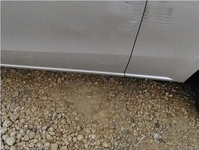
1: Qtr Panel nsr Dented Over 30mm
