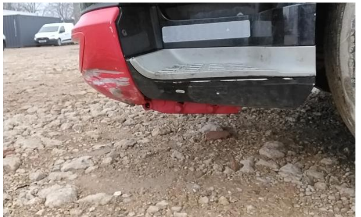
6: Bumper Front Dented With Paint Damage
