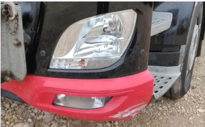
5: Wing nsf Cracked Replace
