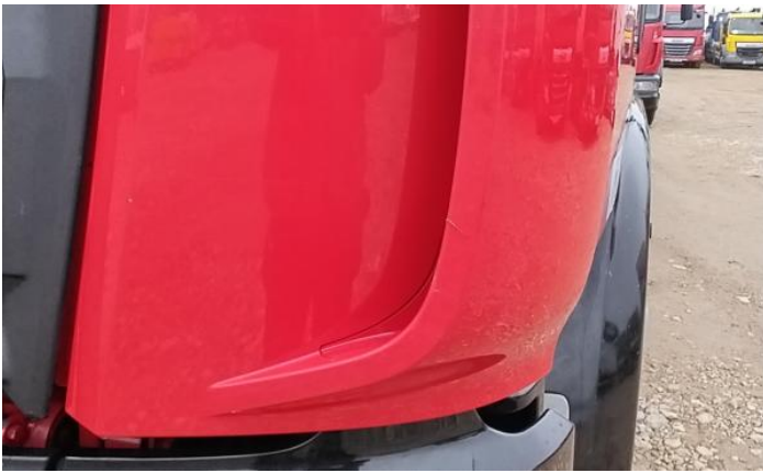
3: Bumper Front Chipped Multiple Chips
