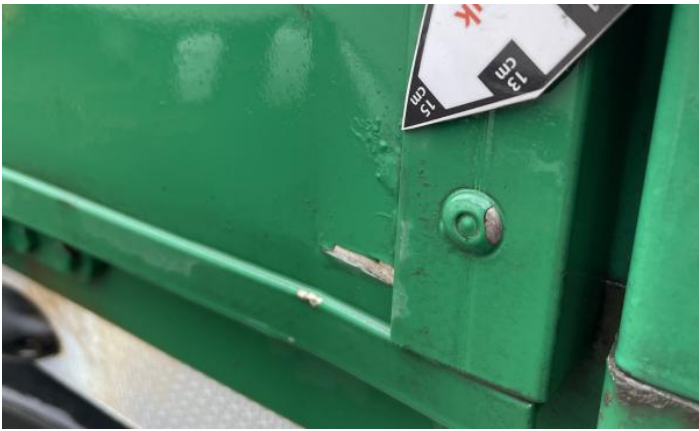
3: Door nsf Scratched Over 25mm Thru Paint
