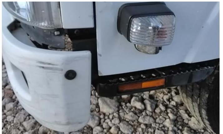
6: Panel Front Scratched Over 25mm Thru Paint
