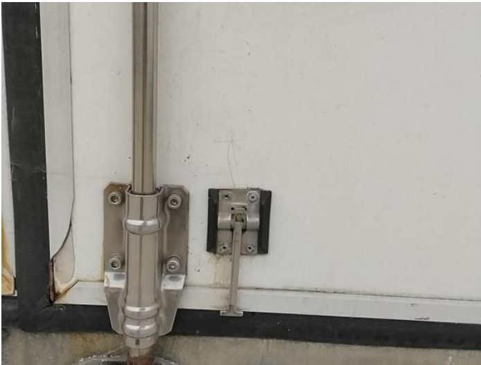
5: Door osr Rusted Over 5mm
