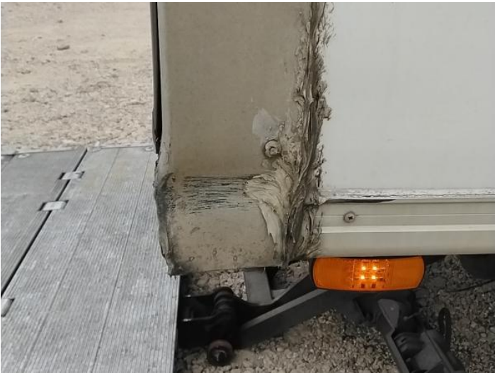
6: Qtr Panel osr Dented Over 30mm
