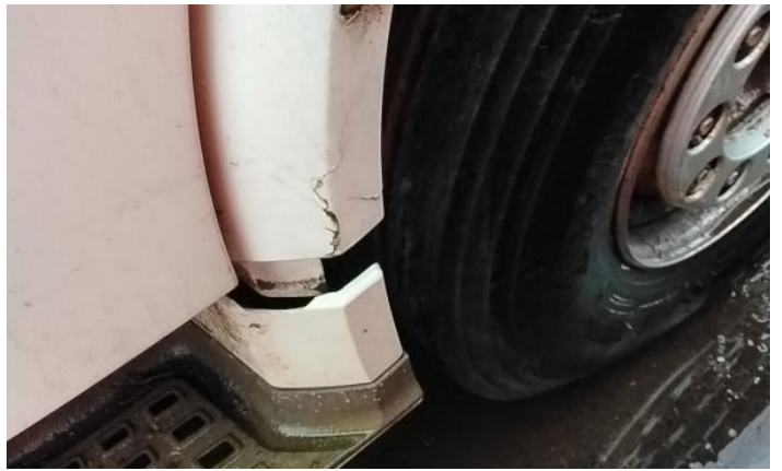
4: Panel Front Scratched Over 25mm Thru Paint
