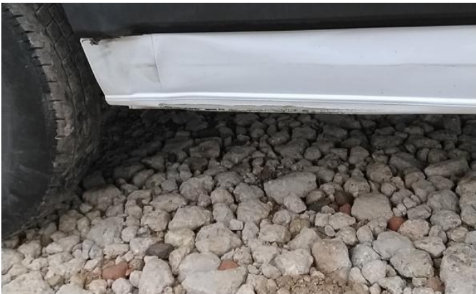
15: Qtr Panel osr Dented With Paint Damage
