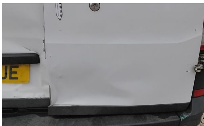
10: Door nsr Dented Over 30% Of Panel
