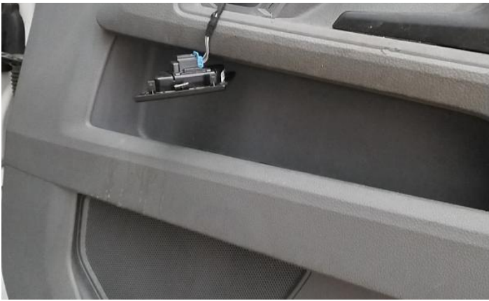
21: Glove Box Lid Broken Replace
