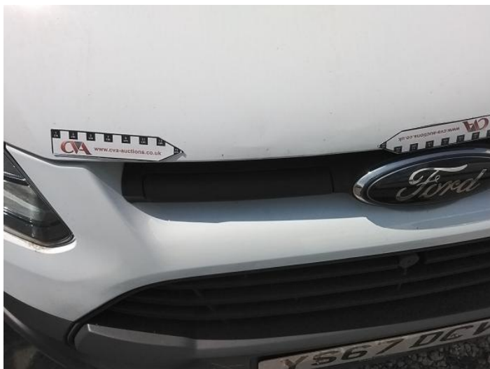
1: Bonnet Dented Over 30mm
