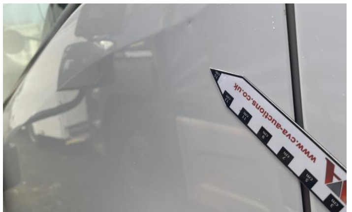
6: Qtr Panel nsr Dented Over 30mm
