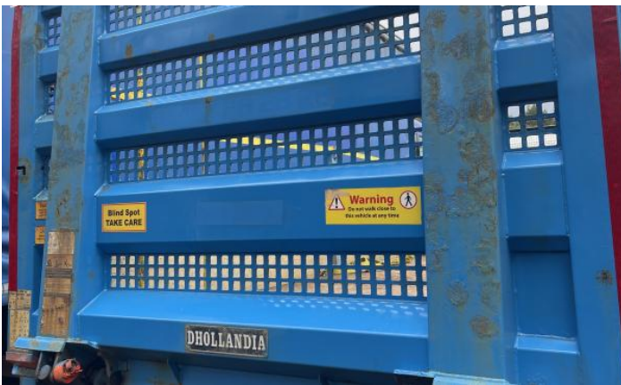
3: Door osf Dented Over 30mm
