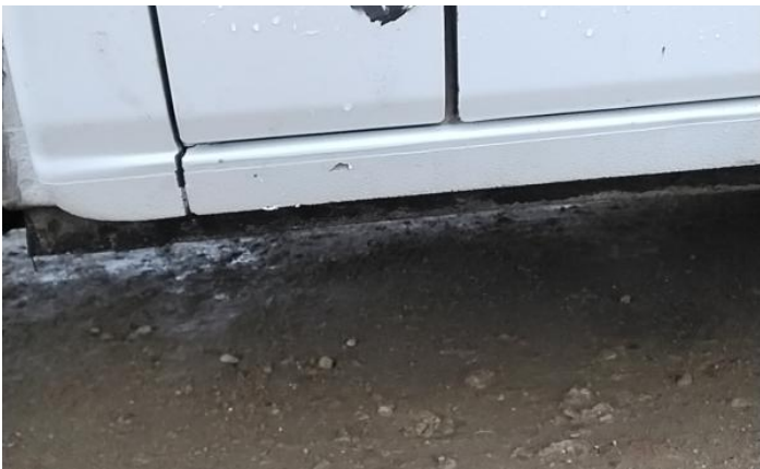
5: B Post ns Scratched Over 25mm Thru Paint
