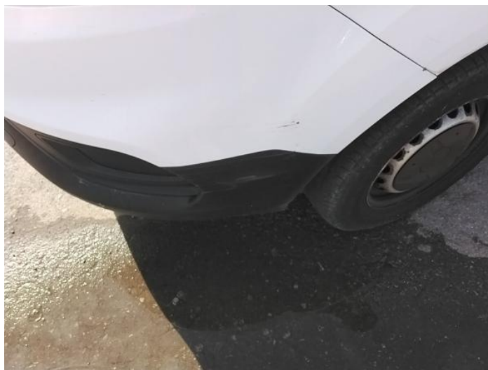
2: Bumper Front Scratched Over 100mm Thru Paint
