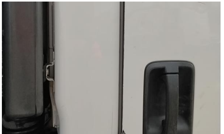
12: Door osf Dented Between 10mm + 30mm
