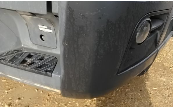
3: Wing Front Arch Extension os Scratched (Painted) Over 25mm Thru Paint
