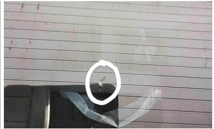
4: Door nsf Scratched UpTo 25mm Thru Paint
