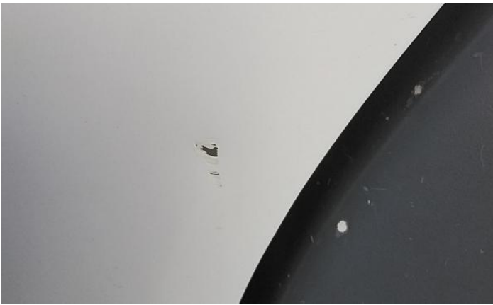
3: Door osf Dented Over 30mm
