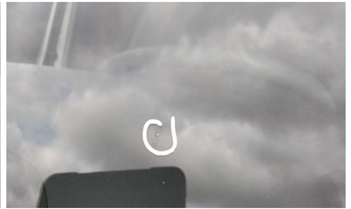
4: Panel Front Chipped Over 5mm
